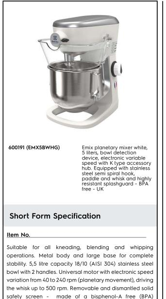
safety screen - made of a bisphenol-A free (BPA) copolyester - activates the raising and lowering of the bowl. Equipped with accessory drive hub type k (accessories are not included). Bowl detction device allows the mixer to switch on only when the bowl and the safety screen are properly installed and positioned together.
